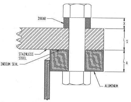
Figure 5-1 Flange joint with Invar washer.
