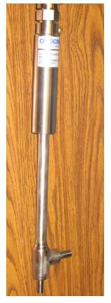
JT Valve Cryocomp ½ inch IPS Designed to be installed inside cryostats Heat Leak to 4.2 K is ~ 1 W
